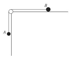
Particles A and B, of masses 0.2 kg and 0.3 kg respectively, are connected by a light inextensible string. The string passes over a smooth pulley at the edge of a rough horizontal table. Particle A hangs freely and particle B is in contact with the table (see diagram).
