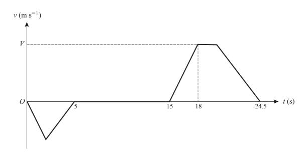
The diagram shows the velocity-time graph for a lift moving between floors in a building. The graph consists of straight line segments. In the first stage the lift travels downwards from the ground floor for 5 s, coming to rest at the basement after travelling 10 m.
